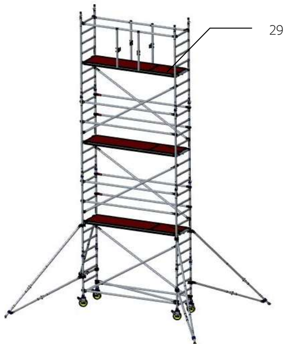
29: Place the platform with hatch (on the 5 th rung from the top), Slide both blow-away protections under the rung.
